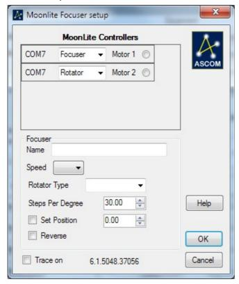
• Use the combo box to set Motor 2 to be a Focuser instead of a rotator and select it:
